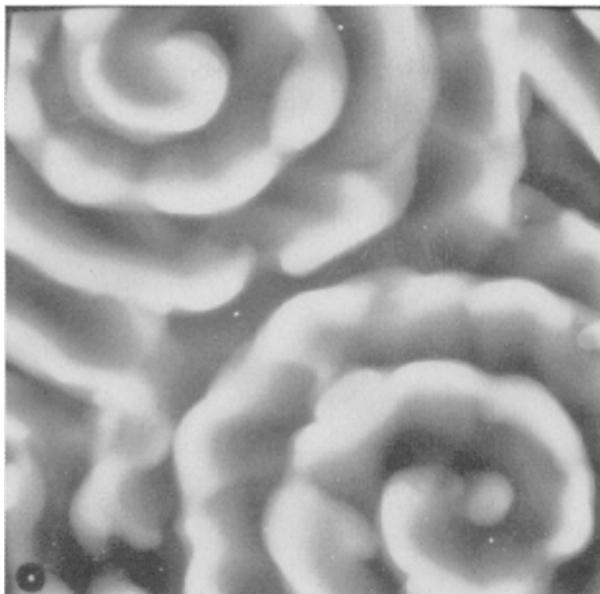
**Fig. 2.** A pair of spiral waves in a liquid BZ layer deformed by natural Marangoni convection. A description of the measurement is given in [15].
