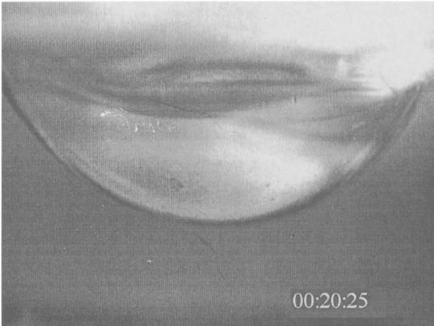
**Fig. 9.** Photograph showing the hanging drop in its initial configuration.
