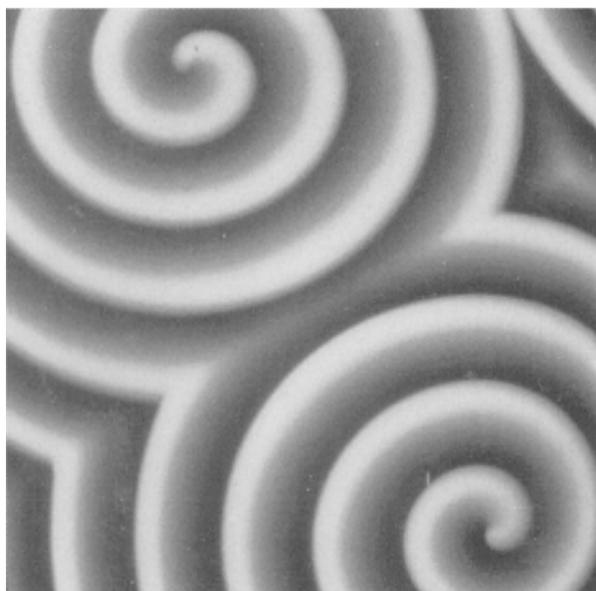
**Fig. 1.** An undisturbed pair of spiral waves in a liquid layer of BZ solution, observed at 490 nm with a 2D spectrophotometer (Image side length: 1 cm)
